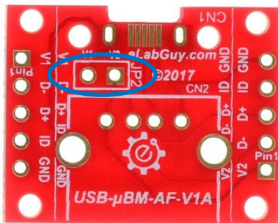
Figure 5: PCB front with open circuit on VCC pin in series
